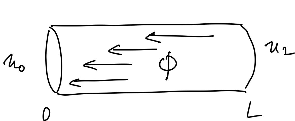
$$\begin{aligned}\phi &= -k_0 \frac{\partial u}{\partial x} \\ &= -k_0 \frac{(u_1 - u_0)}{L}\end{aligned}$$
