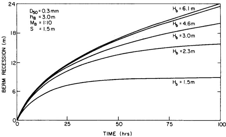
Fig. 7. Effect of wave height on berm recession.
