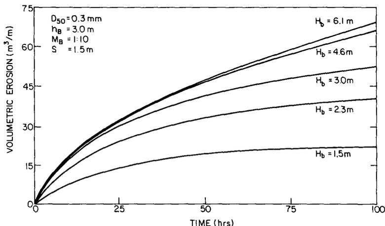
Fig. 8. Effect of wave height on volumetric erosion.
