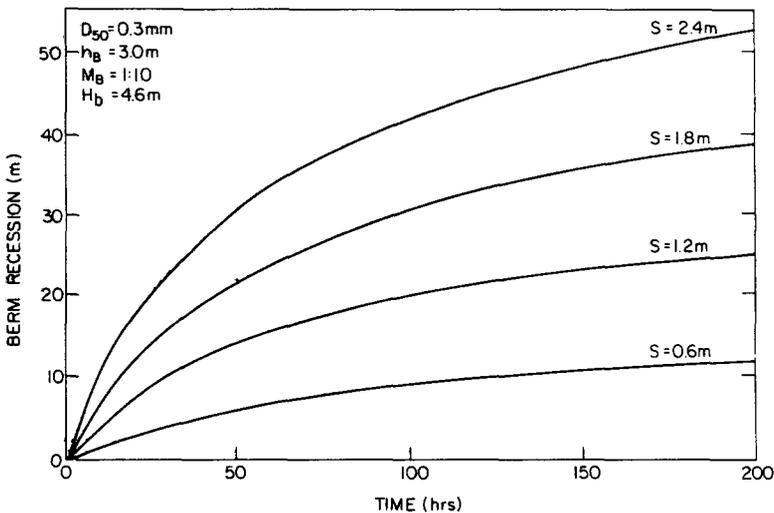
Fig. 5. Effect of static storm surge level on berm recession.
