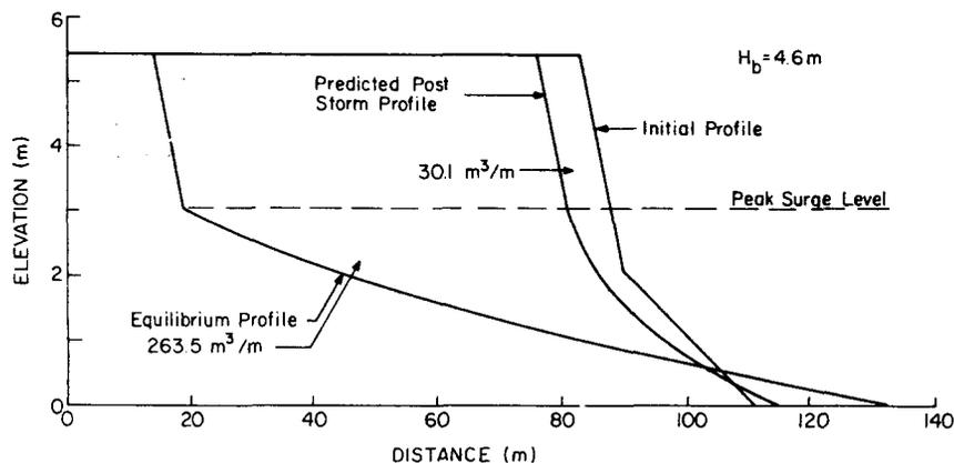
Fig. 18. Comparison of predicted post-storm beach-dune profile to maximum potential erosion associated with peak surge level.
