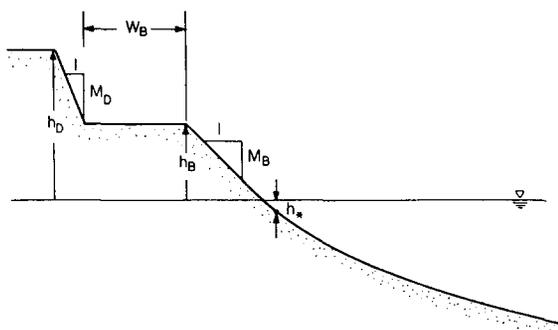
Fig. 2. Schematic dune representation with wide berm.
