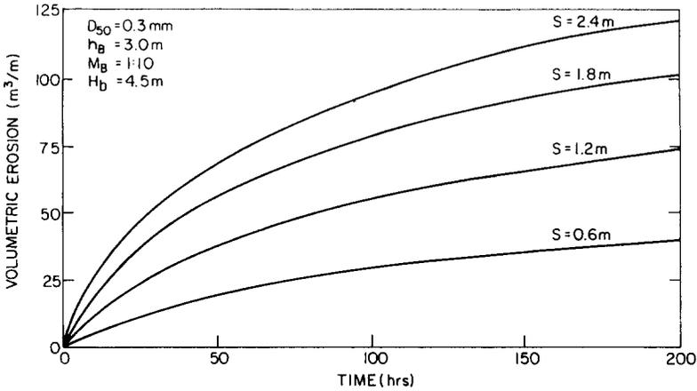
Fig. 6. Effect of static storm surge level on volumetric erosion.
