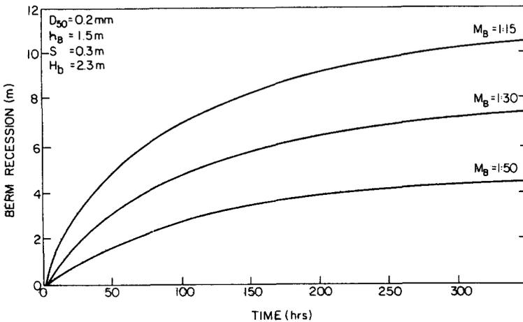
Fig. 10. Effect of beach face slope on berm recession.
