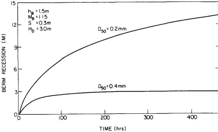
Fig. 9. Effect of sediment size on berm recession.
