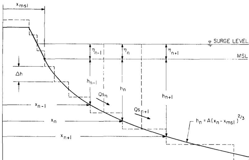
Fig. 1. Model representation of beach profile, showing depth and transport relation to grid definitions.
