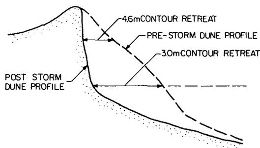
Fig. 15. Steepening of natural dune during erosion.
