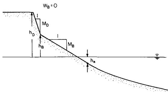
Fig. 3. Schematic dune representation with no berm.
