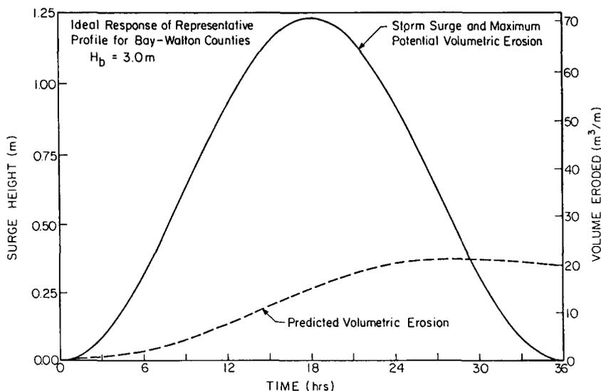
Fig. 13. Effect of storm surge duration on volumetric erosion, thirty-six hour storm surge duration.
