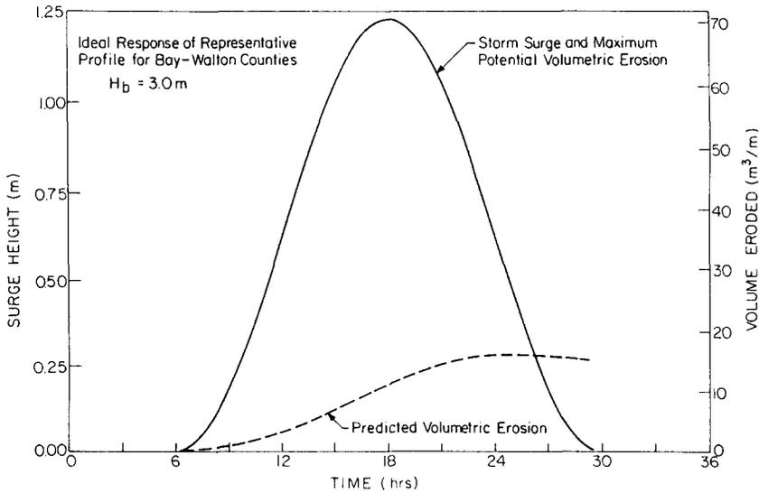
Fig. 12. Effect of storm surge duration on volumetric erosion, twenty-four hour storm surge duration.
