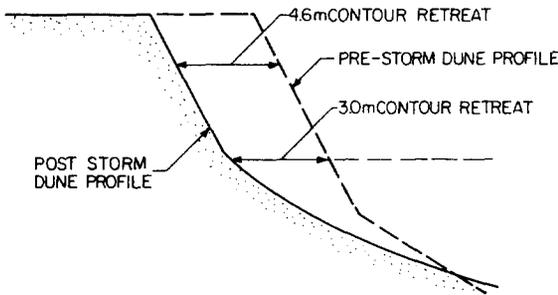
Fig. 16. Uniform recession of schematic dune form.
