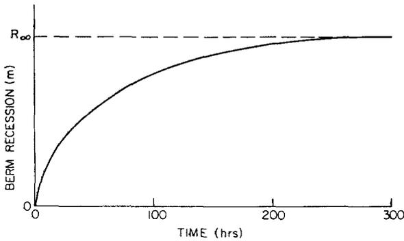
Fig. 4. Characteristic form of berm recession versus time for increased static water level.
