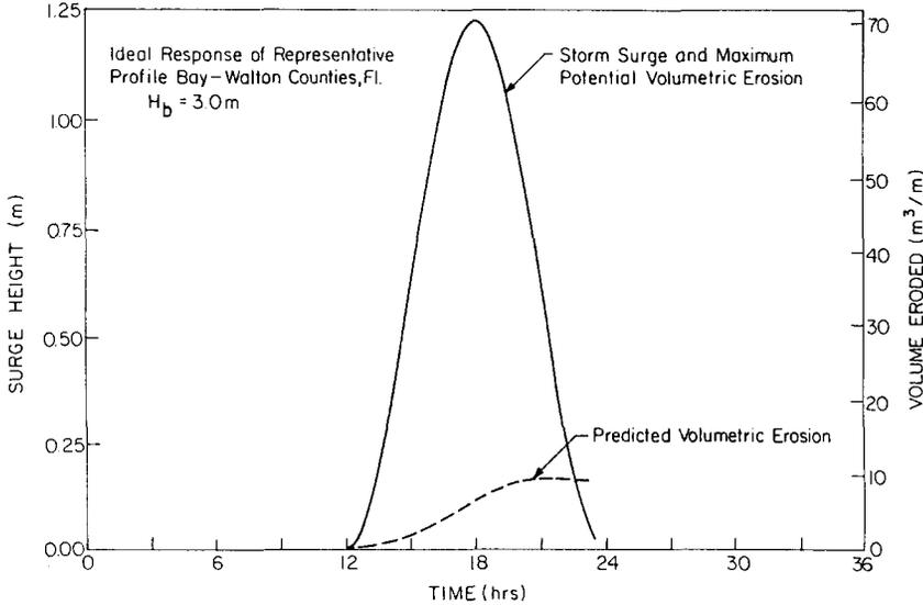
Fig. 11. Effect of storm surge duration on volumetric erosion, twelve hour storm surge duration.
