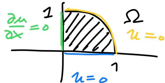
in  $\Omega = \{(x, y), x > 0, y > 0, x^2 + y^2 < 1\}$
