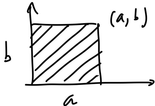
$$\left. \begin{array}{l} u(0, y) = 0 \\ u(a, y) = 0 \\ u(x, b) = 0 \\ u(x, 0) = f(x) \end{array} \right\}$$
