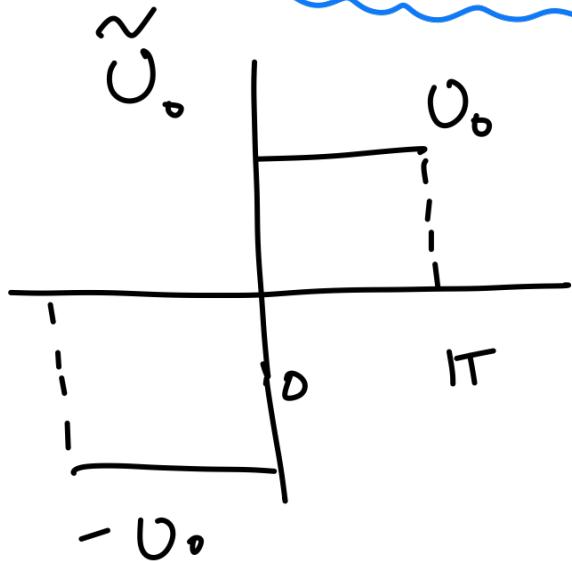
$$\begin{aligned} & \int_{-\pi}^{\pi} \tilde{U}_0 \sin n\theta d\theta \\ &= \int_{-\pi}^{\pi} \sum_{k=1}^{\infty} A_k a^k \sin k\theta \sin n\theta d\theta \end{aligned}$$
